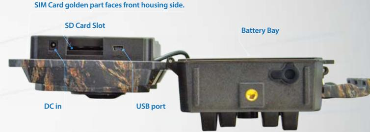
2.3 Figure 3: Internal, Side and Back View
